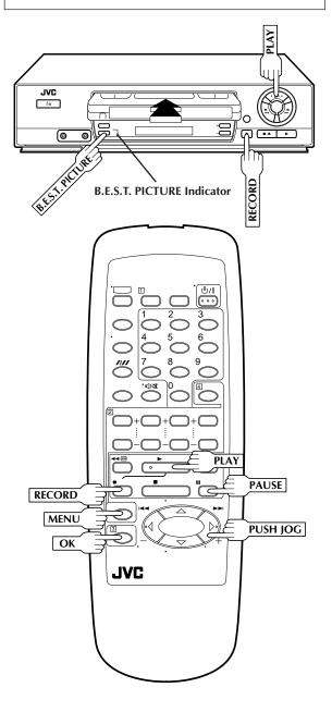
The B.E.S.T. (Biconditional Equalised Signal Tracking) system checks the condition of the tape in use during recording and playback, and compensates to provide the highest-possible recording and playback pictures. The default setting for both recording and playback is "ON".
